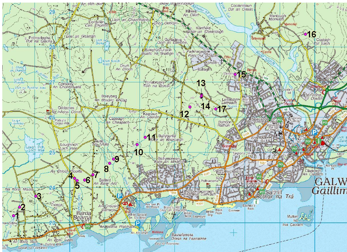
Figure 1 Location Map of Culverts (note reference 11 represents a channel diversion to the northwest of alignment to achieve a single stream crossing at reference 10)
